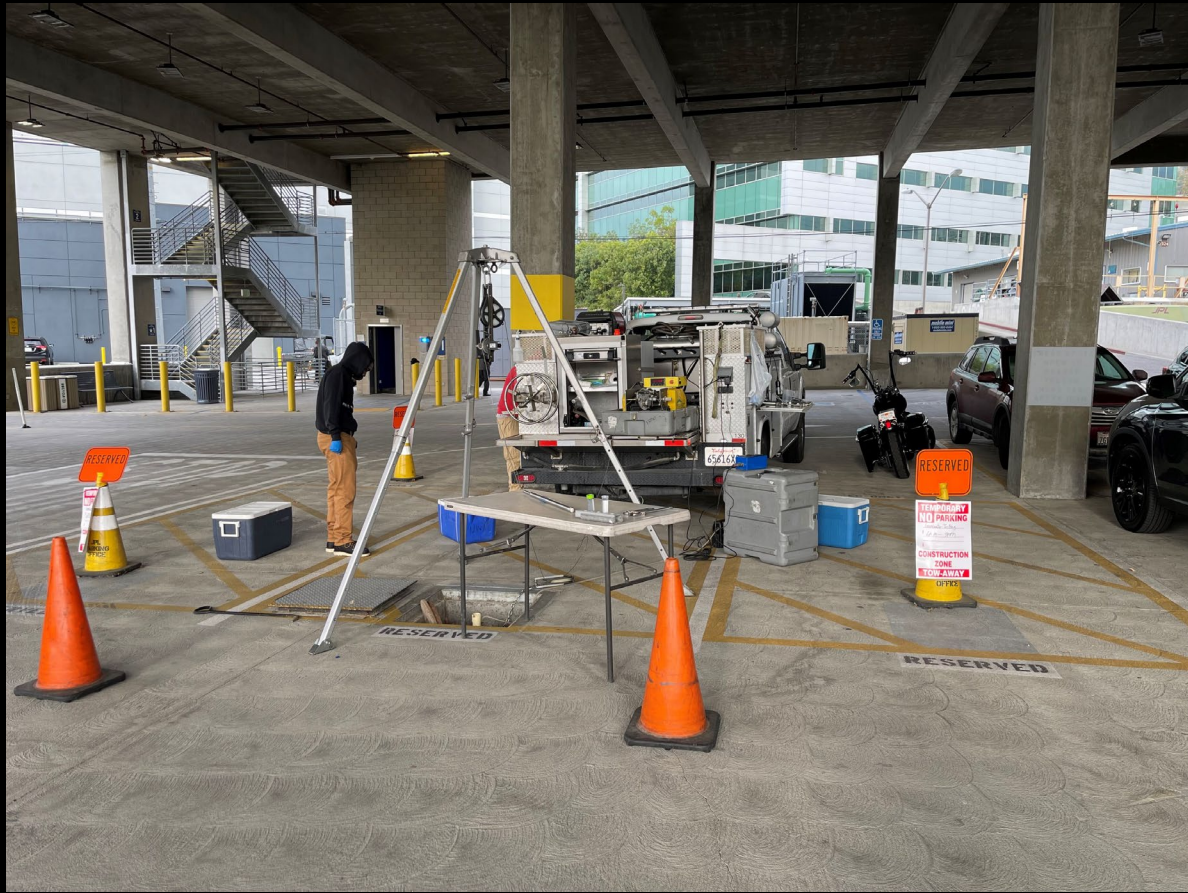
Groundwater Sampling (MW-4)
