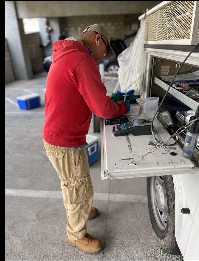
Recording Groundwater Quality Parameters (MW-12)
